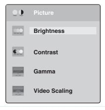
**Brightness**—Adjusts the amount of light in the darkest portion of the picture. Use the lowest brightness setting you are comfortable with to maximize the life of the monitor backlights.
